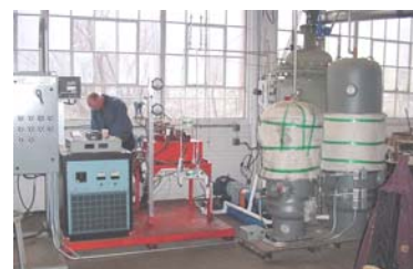
Fig. 13. 50 BBL Test unit for recovery of sub-micron iron catalysts from Fischer-Tropsch wax
