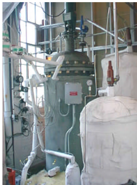
Figure 8. Feed Tank with Mixer on Top. Overflow and Underflow Tanks Are Shown on the Right covered with Insulation.
